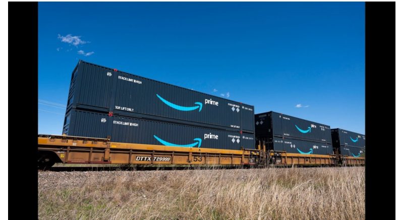
53 ft ribbed car from an IM with Amazon Prime double stack cans.
