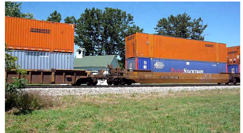
Two 53 ft double stack IM cars. Ribbed car on the left much more likely to be rideable than smooth car on the right.
